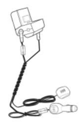
Be sure to choose a location carefully by taking notice of how doors and trunks open and close, as well as how seats move when they are adjusted so you can be certain there is ample clearance provided for the cables.
